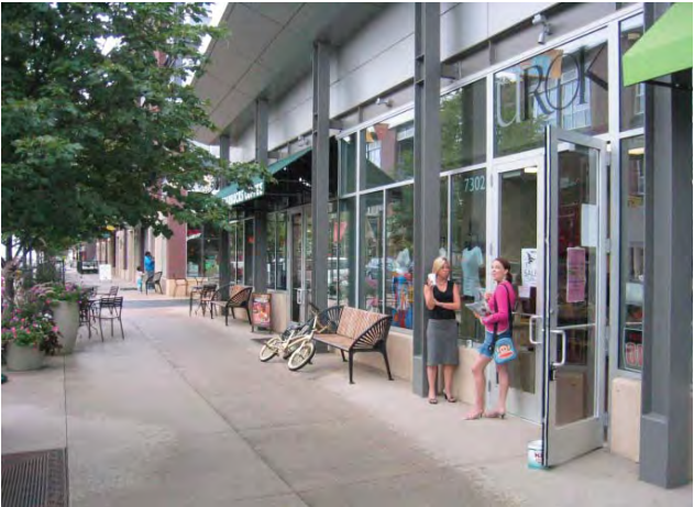
A five-foot minimum clear path of travel on sidewalks ensures a comfortable and accessible environment for all users.
