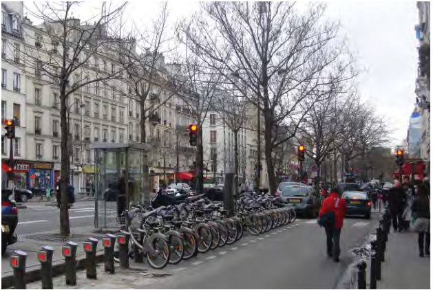
Side access streets allow for slow-moving and local destination-bound traffic to access buildings and properties between intersections.
